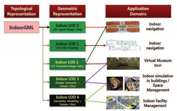
Figur 6. Examples of Indoor Applications Based on Proposed Indoor LOD Model
