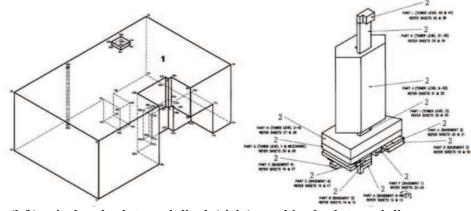
Figure 11. a (left) a single-valued stepped slice b (right) a multi-valued stepped slice
