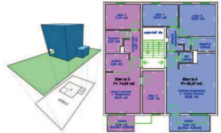
Figure 4. Property on the cadastral map and presentation of parts (separate and common) per floor
