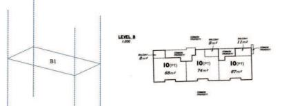
Figure 9. a (left) 2D spatial unit b (right)/spatial units defined by the structure (the buildings walls)
