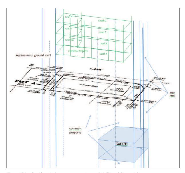
Figure 9. Side view of result after corner truncation and definition of Easement A
