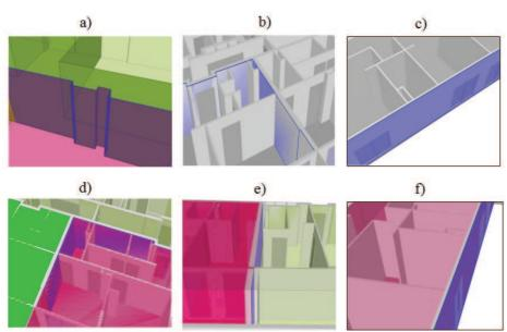
Figure 9. Visualization of structural boundaries in BIM models: a) Visually ambiguous boundary type in legal model b) Internal boundary in physical model c) External boundary in physical model d) Internal boundary in integrated model e) Median boundary in integrated model f) External boundary in integrated model
