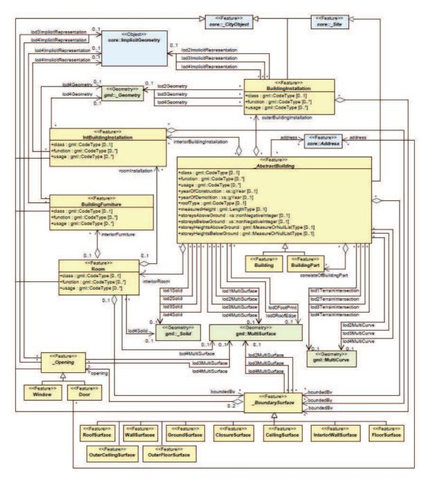
Figure 2. Building model of CityGML, adapted from (Groger et al, 2012, p. 63)
