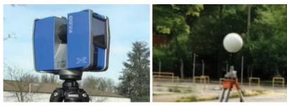
Figure 9. a) Terrestrial laser scanner Faro Focus3D x 330 (left) and b) spherical target positioned on the tripod with tribrach (right)
