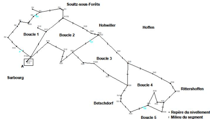
Fig. 5 The leveling network connecting the 13 gravimetric sites of Soultz network (5 loops) and comparison of height difference for consecutive section during the period 2014 – 2015 (after Ferhat et al. 2015).
