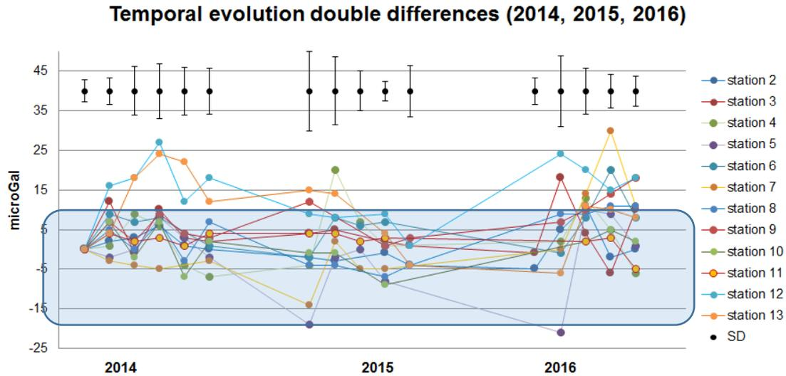
Fig. 4 Example of gravity double differences in 2014, 2015 and 2016 at the 12 sites of Soultz network (stations 2 to 13). The blue area is the  $\pm 2 \sigma$  uncertainty band computed from the uncertainties in the measurements and processing of all surveys.
