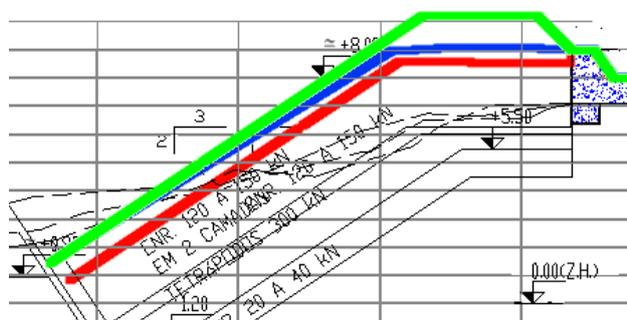
Fig. 19 Three profiles of the project. See text for explanation of the colors used. In the graph each rectangle has 1 meter height
