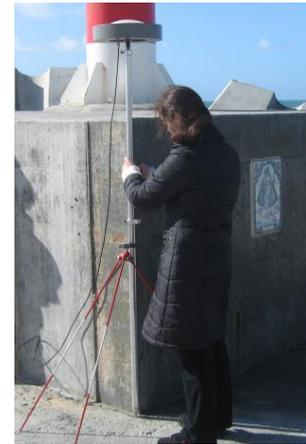
*Fig.10 Coordinating a point by GNSS*
