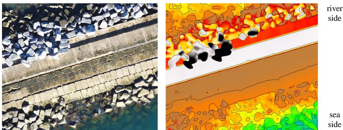
Fig. 12 Detail of Portimao east breakwater: orthomosaic and colored DSM with contour lines
