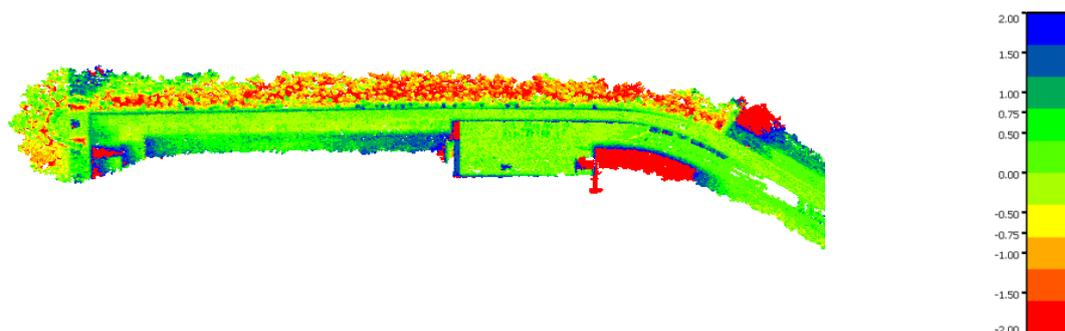
Fig. 17 Differences between two point clouds: project and photo survey. Scale unit: meter
