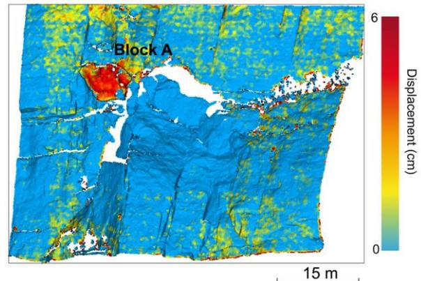
Figure 9. Case 2. Degotalls wall. Result of TLS monitoring. Example of movement detection comparing TLS campaigns.
