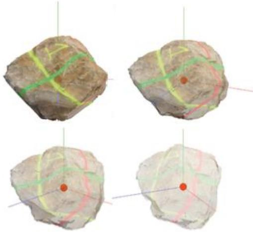
Figure 3. Site1, Block 1 3D model, where the centre of mass is positioned from four points of view.
