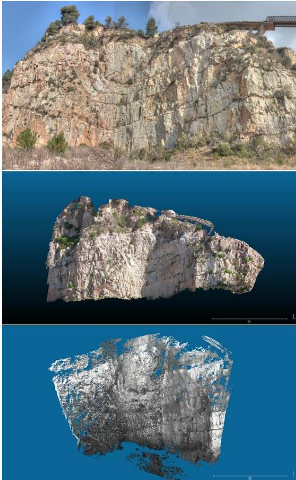
Figure 5. From top to bottom, picture, photogrammetric model and TLS model of the Olorda quarry
