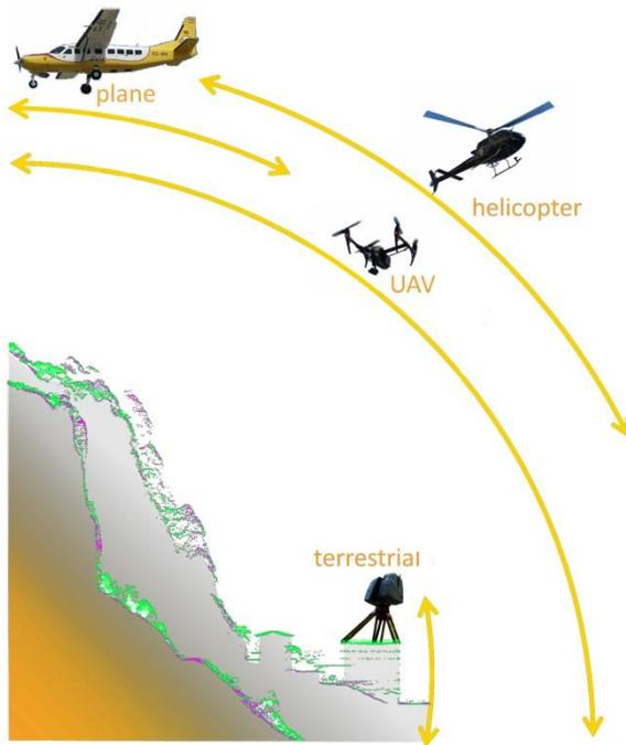
Figure 1. Different geomatic techniques and platforms to capture 3D information (modified from Janeras et al., 2018a).
