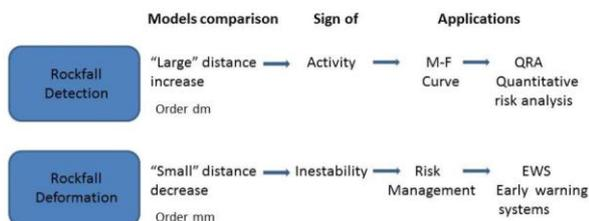
Figure 6. TLS role in Rockfall Detection and Deformation
