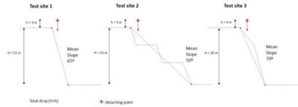
Figure 2. Sections of the different test site in quarries.
