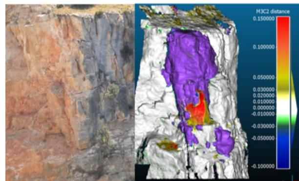
Figure 7. TLS, Case 1. Left: picture of a rockfall detected between two campaigns. Right: volume loss of 28 m<sup>3</sup> (purple) and displacement of the rock (red).
