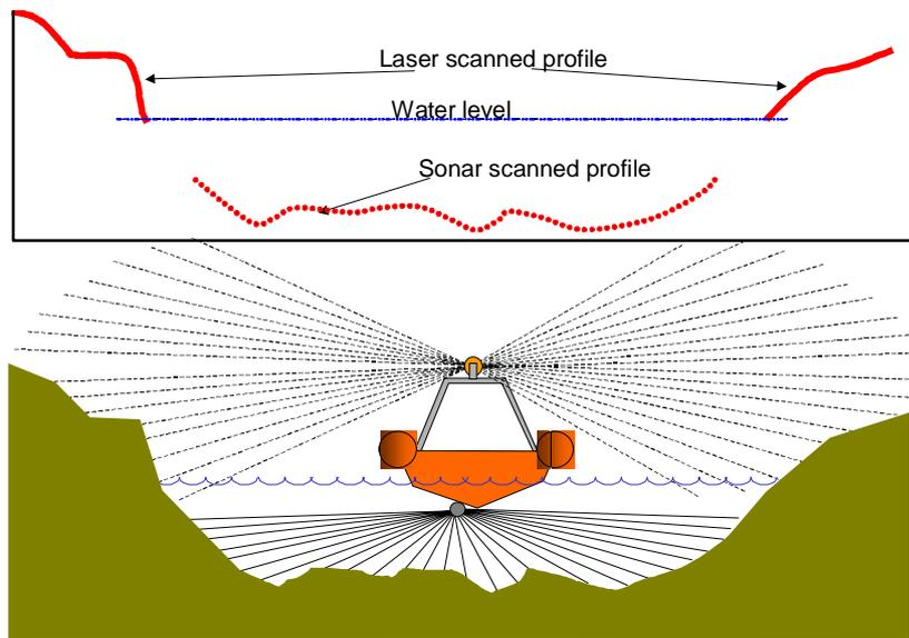
Fig 2. Combined Acoustic and Laser scanned Profile
