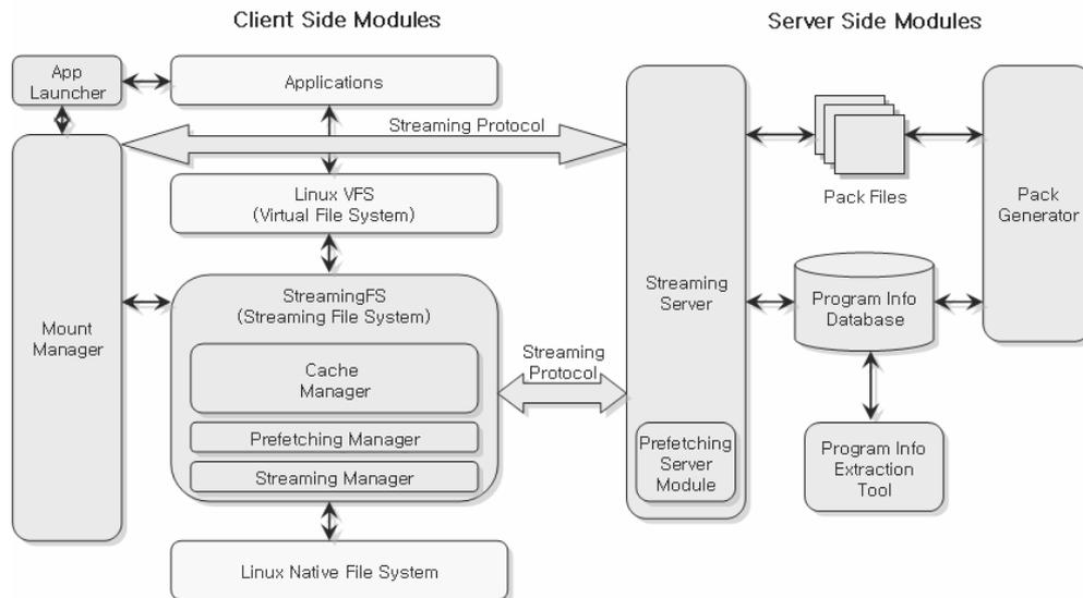
**Figure 4. System Architecture of Streaming Transmission Which is Tightly Coupled to Operating System**
