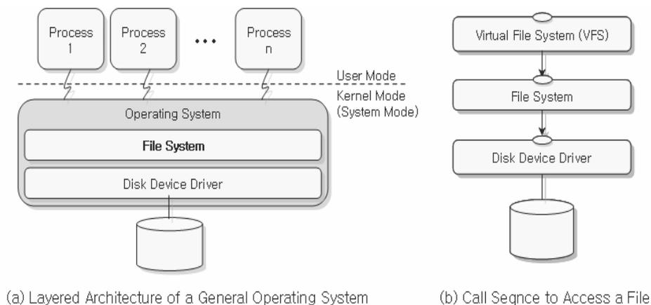
**Figure 1.** General Architecture of an Operating System
