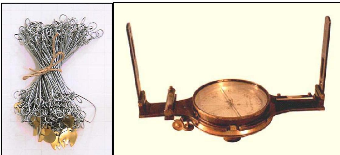
**Figure 1** – Gunter's Chain (left) and Surveyor's Compass or Circumferentor used in early surveys (Courtesy [www.gmat.unsw.edu.au/currentstudents/ug/projects/f\\_pall/html/index.html](http://www.gmat.unsw.edu.au/currentstudents/ug/projects/f_pall/html/index.html) School of Surveying and Spatial Information Systems, Virtual Surveying Instrument Collection).
