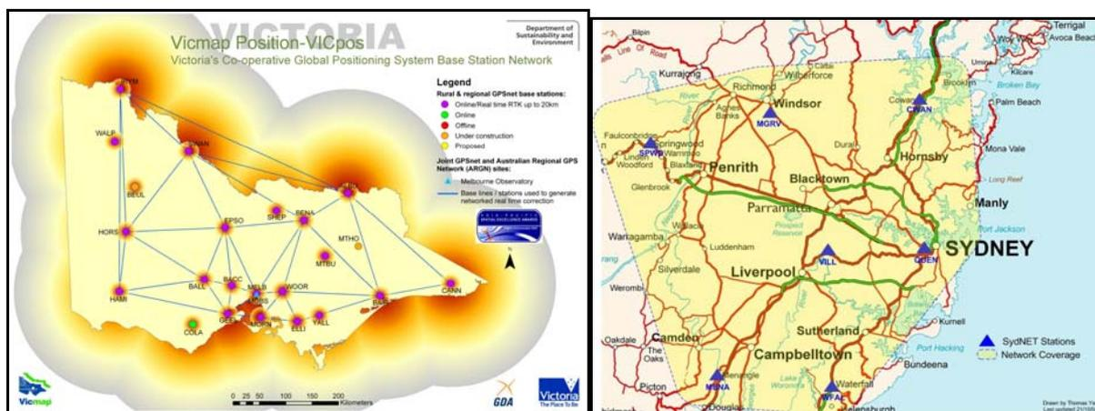
**Figure 3** – a) The VicPos sub-metre service across Victoria and MelPos 2cm service focussed around Melbourne bottom centre of figure (courtesy Dept of Sustainability and Environment, Victoria) and b) SydNet servicing the Sydney basin region.
