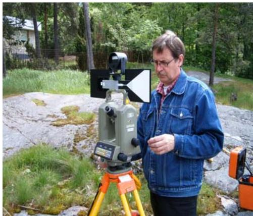
**Figure 4.** Enlarged target used in water crossing tests in Otsolahti.
