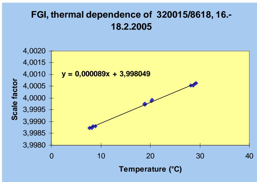
**Figure 2.** Thermal dependence of scale factor.
