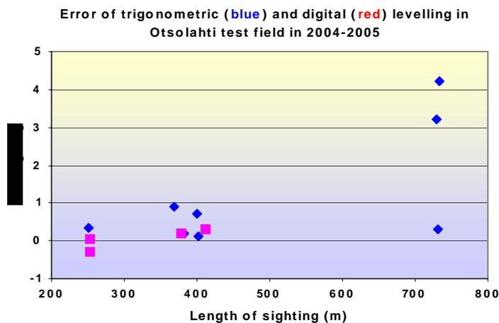
**Figure 6.** The accuracy of the water crossing test measurements
