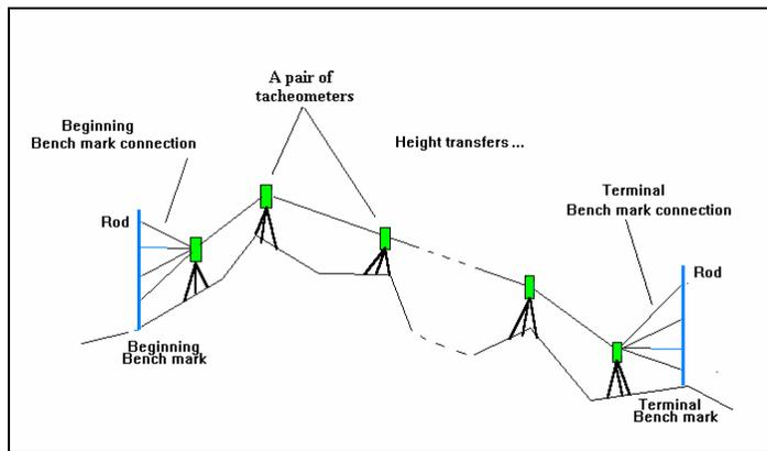
**Figure 3.** Principle of trigonometric levelling
