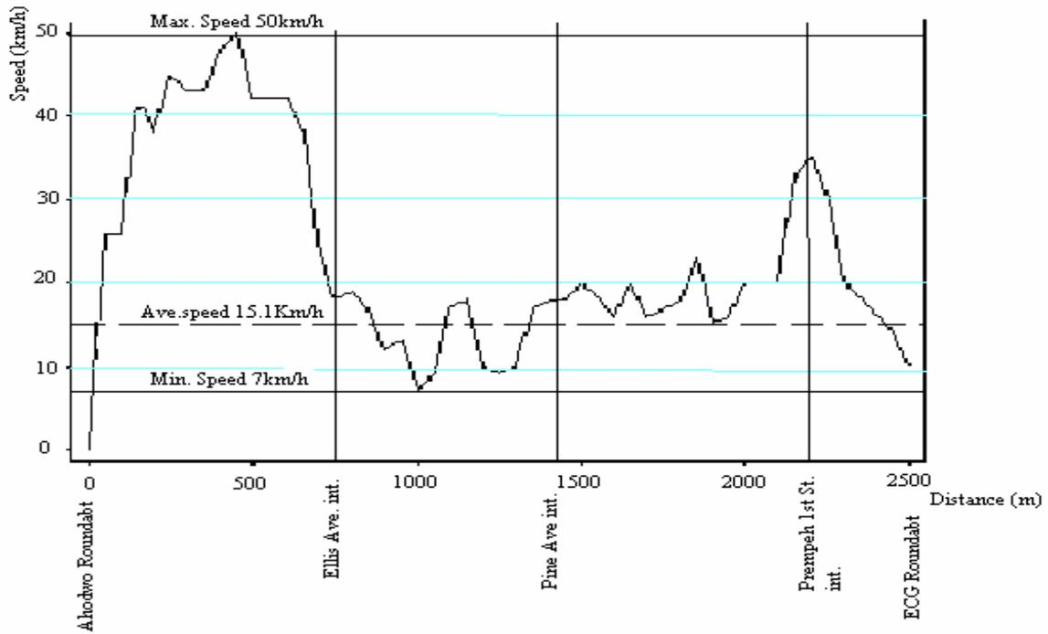
**Fig.2** Speed Profile from a GPS file for Harper road during AM period towards the CBD.
