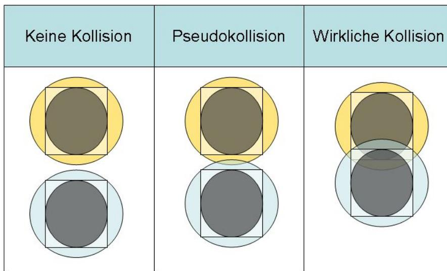
**Fig.1:** Test of centre spacings to discriminate between the 3 different collision cases
