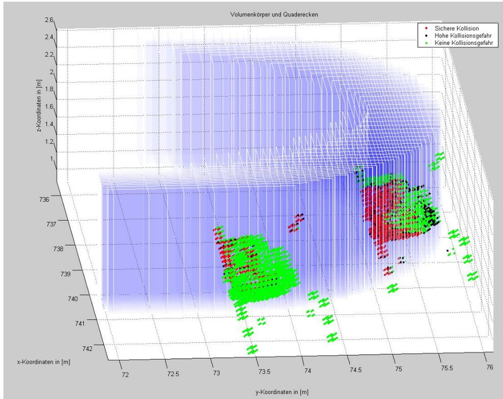
**Fig.5:** Space of impact along a curved section with intentional severe collisions
