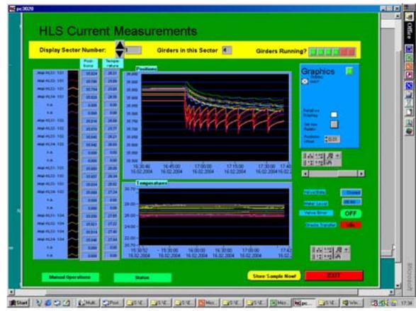
**Fig. 7:** Graphical interface, showing data of the refilling process.
