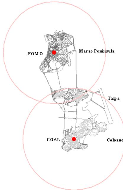
**Figure 1:** 5km buffer zone of the GPS reference stations
