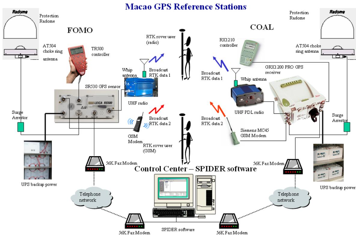
**Figure 2.** The Structure of Macao GPS Reference Stations
