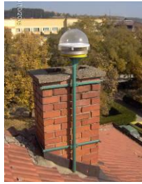
Fig. 8: Type 2 – Pedestal on the metal console
