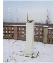
Fig. 9: Type 3 – Pedestal on the column
