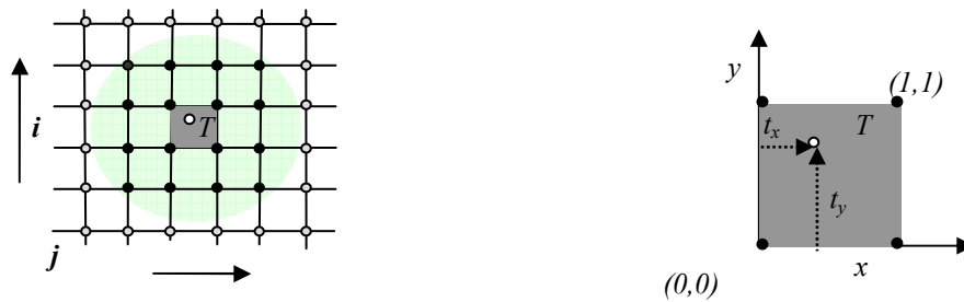
Figure 4. Geometrical scheme showing 16 nodes utilized for interpolation (bold black) (left), with point T located within inner cell (right).
