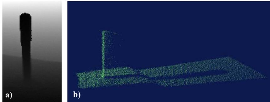
**Figure 2:** Object appearance in the range panorama and its equivalent representation in the 3D point cloud. Neighborhood for any point in the scan can be easily drawn from the image by directly accessing its neighboring pixels.
