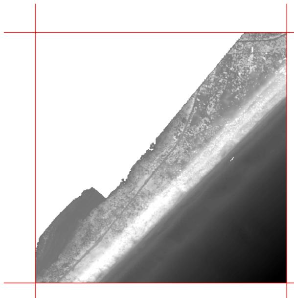
Contour files were created by firstly stitching together each 2km tile into an overall area mosaic. This file was subsequently run through three stages of filtering, which smoothes the data by reducing local variation using a 3 x 3 neighbourhood with a mean statistic type. Contours were created for the entire area at a 1m interval, and clipped using the 2 km tile boundaries. The contours were provided to UTM on the AHD. The following image shows the contours at the Snowy River estuary.
