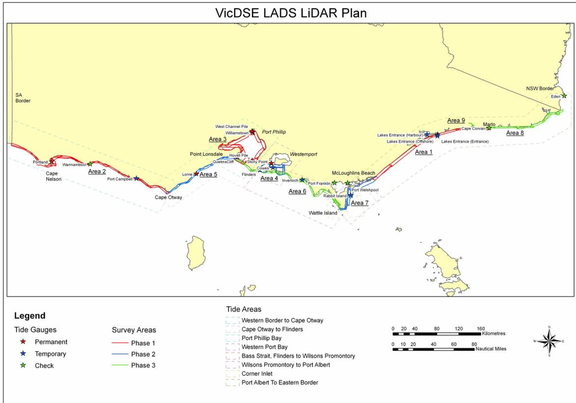
This approach ensured that the surveys were progressed in an order corresponding to the VicDSE priorities. It further ensured alternate areas were available on the west coast, east coast and in a sheltered bay during each phase, in the event of poor environmental conditions. It also followed the important survey maxim of divide and conquer, which enabled areas to be completed progressively, in lieu of trying to survey the entire coast as a single activity.
