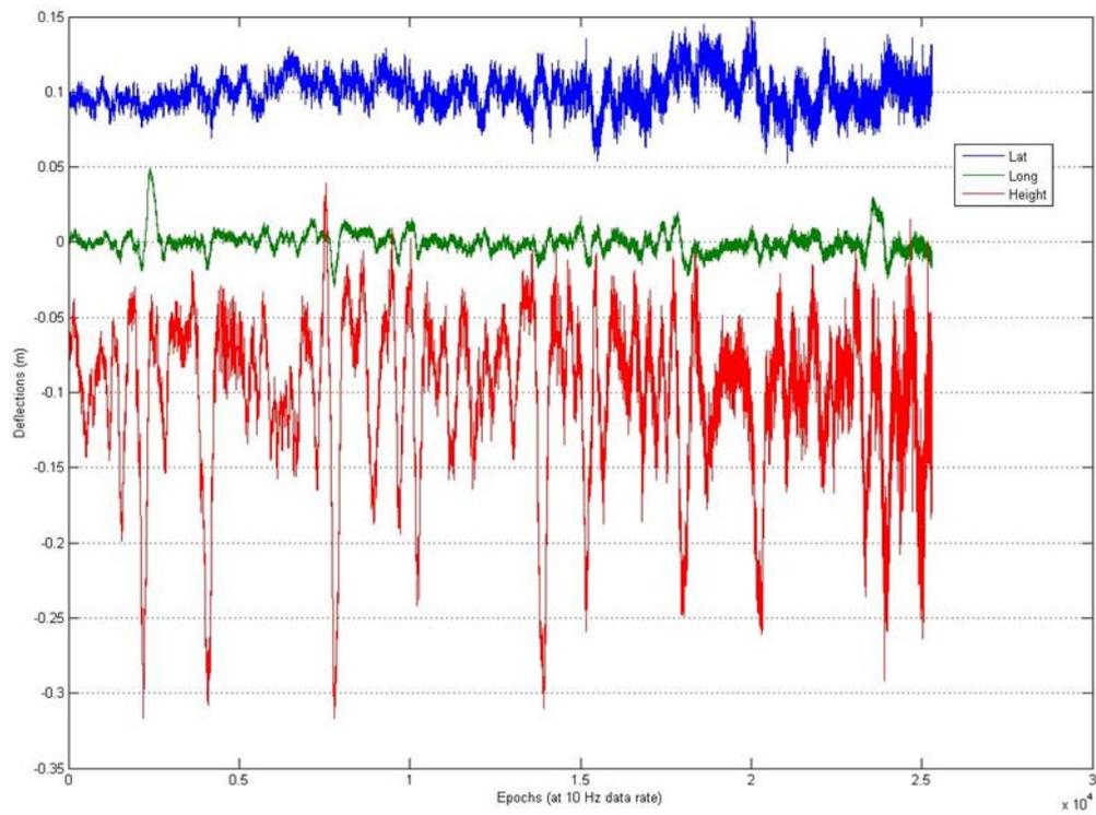
Figure 6. Deflections at point A from 13:09:45 to 13:51:55.
