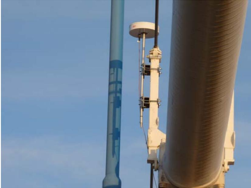
Figure 5. GNSS choke ring antenna located on the suspension cable.
