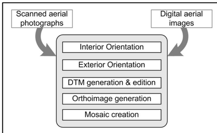
Figure 1. Orthoimage generation process
