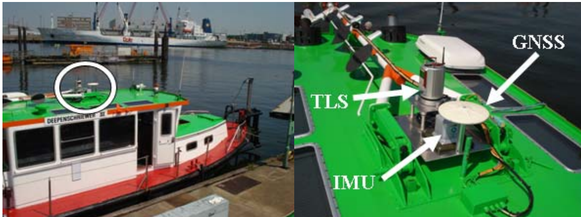
Figure 3: Installation of sensors on board the “Deepenschriewer III”
