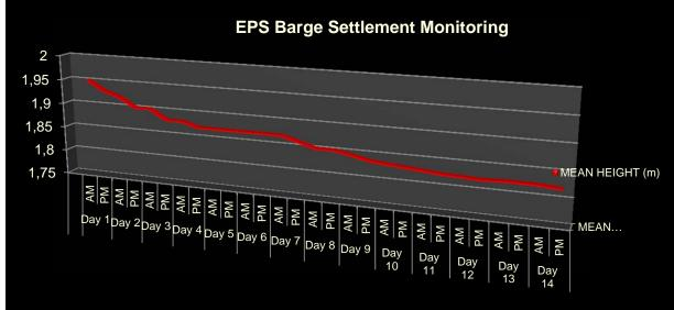
Fig 9: The graph shows the EPS Barge Settlement Monitoring Trend on Location
