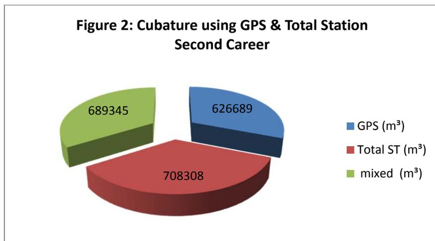
Because of the considerable difference between the results of GPS survey and total station survey, we combined GPS with total Station surveys to get a mixed survey. We can therefore consider the results of the mixed cubature survey as a reference.
