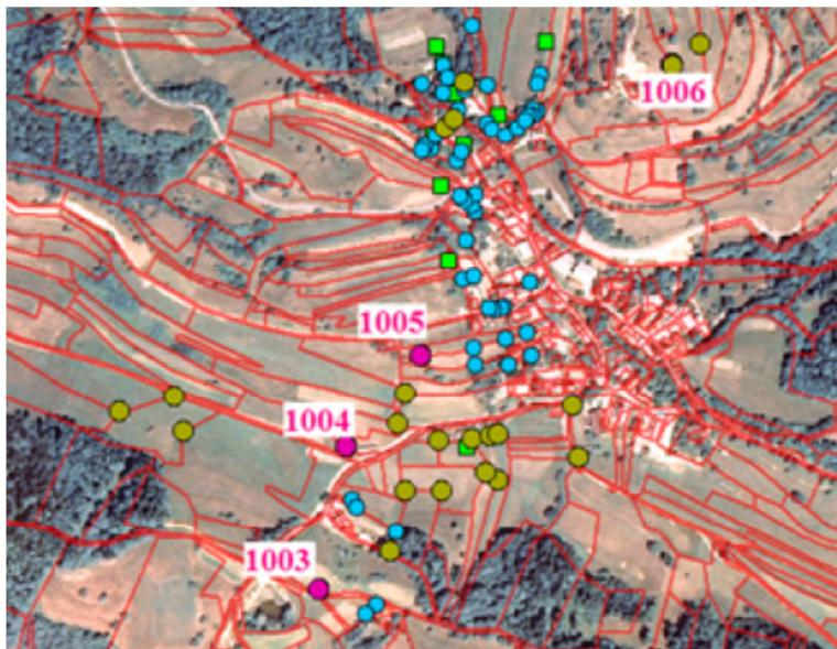
Figure 2: Cadastral index map (red lines) on orthophoto with the identical points: boundary marks of cadastral survey for the 19<sup>th</sup> century (green points), boundary marks of survey in the 20<sup>th</sup> and 21<sup>st</sup> century (blue points), and geodetic points (violet points).
