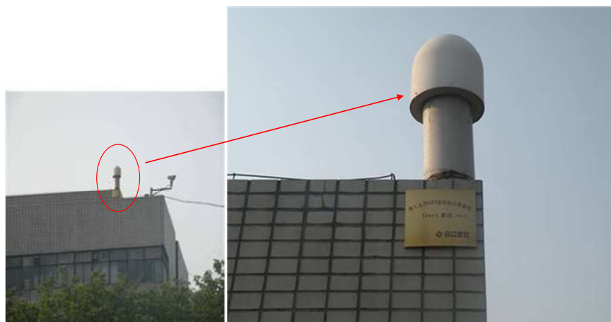
Fig. 1 CDUTCORS base station
