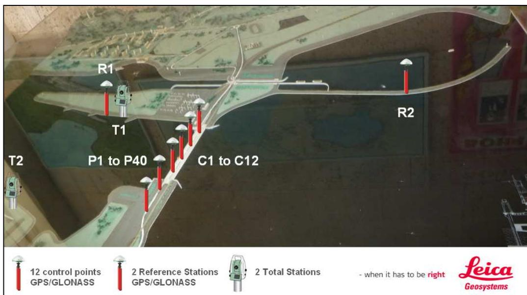
Fig 13: Design with two GNSS Reference Stations – Accuracy is meeting and exceeding the specifications.
