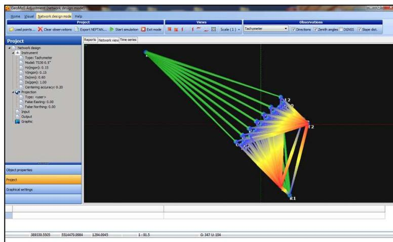
In that simulation mode the size and direction of the error ellipsoids are indicators of how the design could impact on the final coordinates accuracy.
