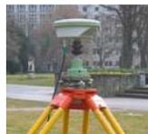
>20,000€, geodetic GPS receiver, dual-frequency
