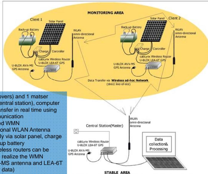
2 clients (rovers) and 1 master (reference, central station), computer raw data transfer in real time using WLAN communication
