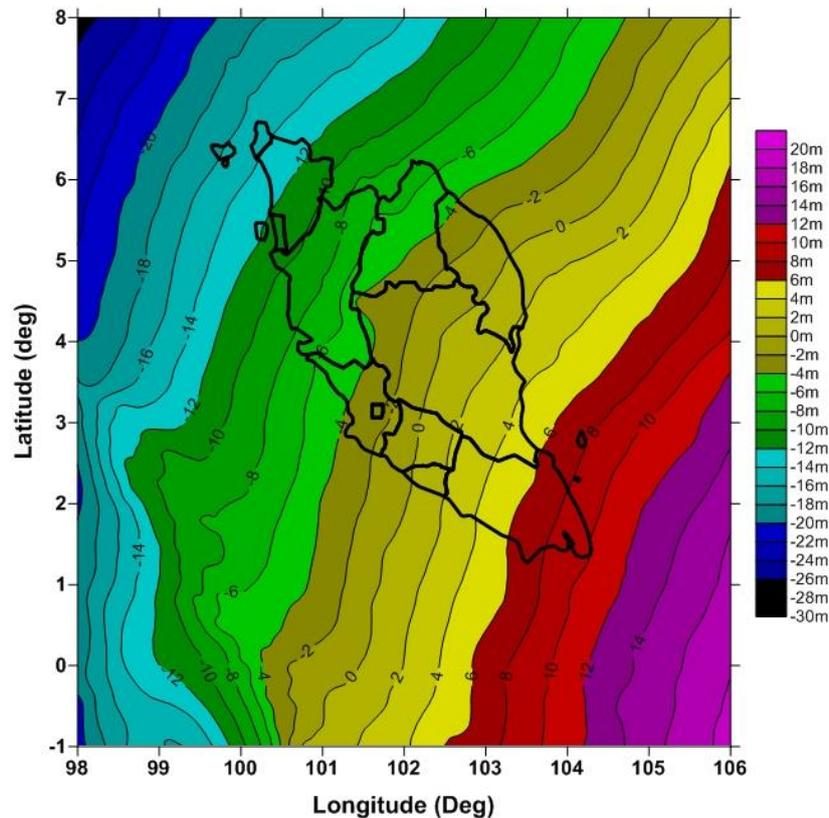
**Figure 3.** 1'x1' arc minute Gravimetric geoid model constructed
