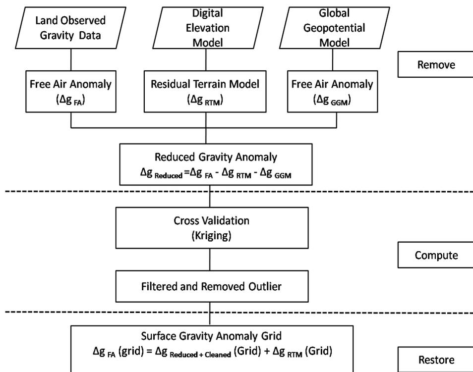
**Figure 2.** Schematic diagram for detecting developed surface gravity anomaly using combination R-C-R and Cross Validation
