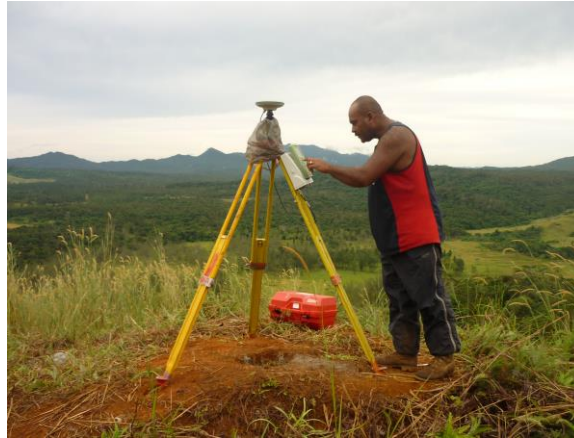
Surveyors operating GPS instrument on third order control monument.
