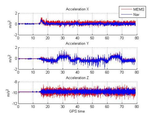
Figure 4: MEMS INS performance tests - accelerations.
