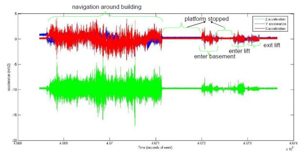
Figure 7: Qualitative information extracted from noisy MEMS data
