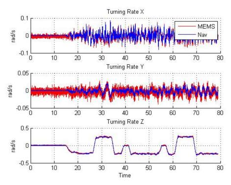
Figure 5: MEMS INS performance tests - turning rates.
