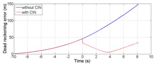
Figure 10: The performance of dead reckoning with and without CIN.
