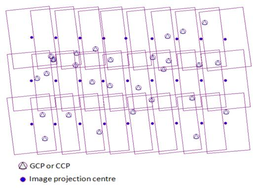
Figure 3: The vertical Pictometry images block showing the distribution of control points and images projection centres.
