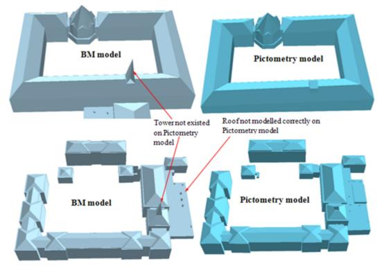
Figure 7: Qualitative comparison between the UltraCamD 3D models (BM) and the vertical Pictometry 3D models for Nottingham University main campus.
