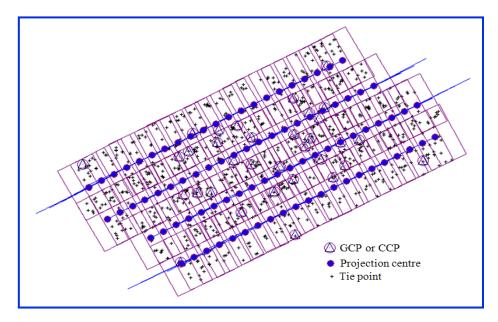
Figure 2: UltraCamD images block showing images footprint, distribution of GCPs and tie points, and camera x-axis.
