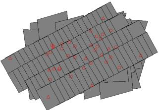
Figure 6: The combined UltraCamD and oblique Pictometry images footprint after performing AT
