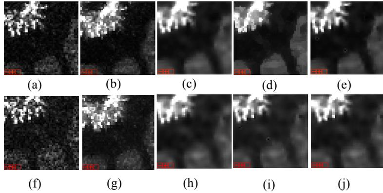
Figure 5. Zoom images of Algiers region. (a) Original *Span*, (b) Lee *Span*, (c) SSC *Span*, (d) Turbo Lee *Span*, (e) Turbo SSC *Span*, (f) Original  $|HH \cdot VV^*|$ , (g) Lee  $|HH \cdot VV^*|$ , (h) SSC  $|HH \cdot VV^*|$ , (i) Turbo Lee  $|HH \cdot VV^*|$ , (j) Turbo SSC  $|HH \cdot VV^*|$ .
