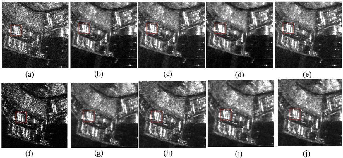
Figure 6. images of Munich region. (a) Original *Span*, (b) Lee *Span*, (c) SSC *Span*, (d) Turbo Lee *Span*, (e) Turbo SSC *Span*, (f) Original  $|HH \cdot VV^*|$ , (g) Lee  $|HH \cdot VV^*|$ ,
