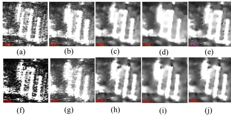
Figure 7. Zoom images of Munich region. (a) Original *Span*, (b) Lee *Span*, (c) SSC *Span*, (d) Turbo Lee *Span*, (e) Turbo SSC *Span*, (f) Original  $|HH \cdot VV^*|$ , (g) Lee  $|HH \cdot VV^*|$ , (h) SSC  $|HH \cdot VV^*|$ , (i) Turbo Lee  $|HH \cdot VV^*|$ , (j) Turbo SSC  $|HH \cdot VV^*|$ .
