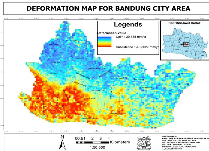
**Figure 4. Deformation map from PS-InSAR processing in Bandung city area.**
