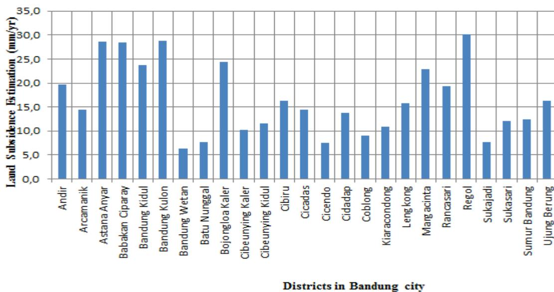
**Figure 6. Land subsidence value estimation in Bandung city from 12 ALOS PALSAR images with PS-InSAR technique**
