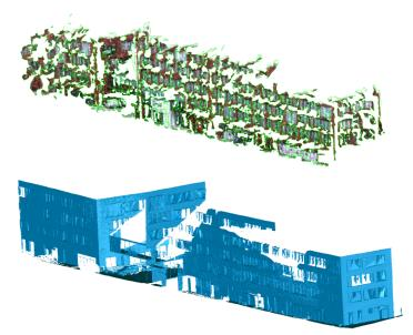
Figure 6Compare the point cloudsfrom the camera sequence (above) and a terrestriallaser scan (below)
