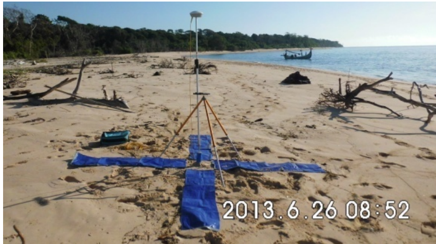
Figure 3. Premark and GCP measurement
