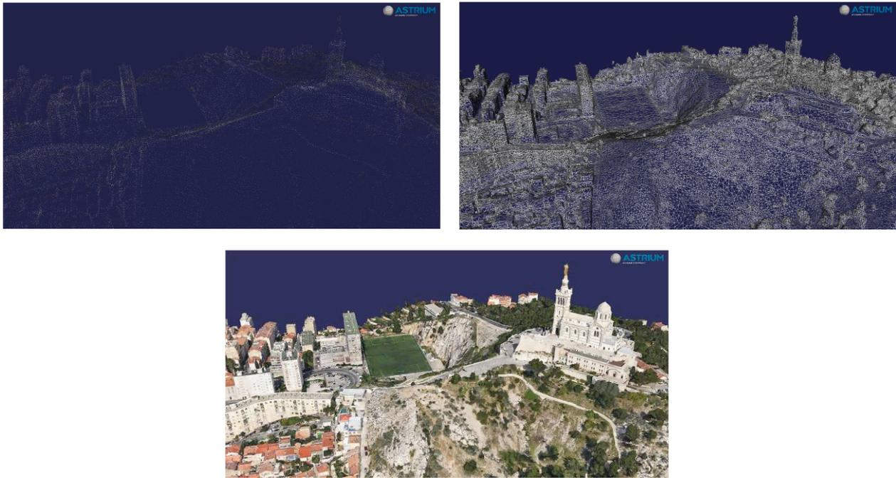
**Figure 2:** From cloud of 3D points to textured 3D Mosaic automatically processed
