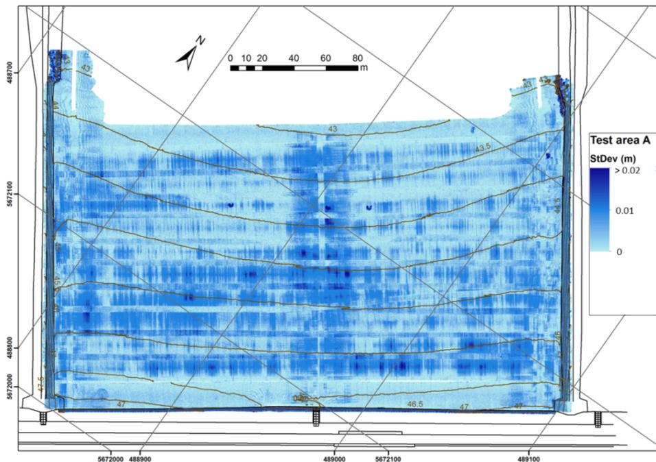
Figure 5: Standard deviation map of the MTLS data (per  $dm^2$ )
