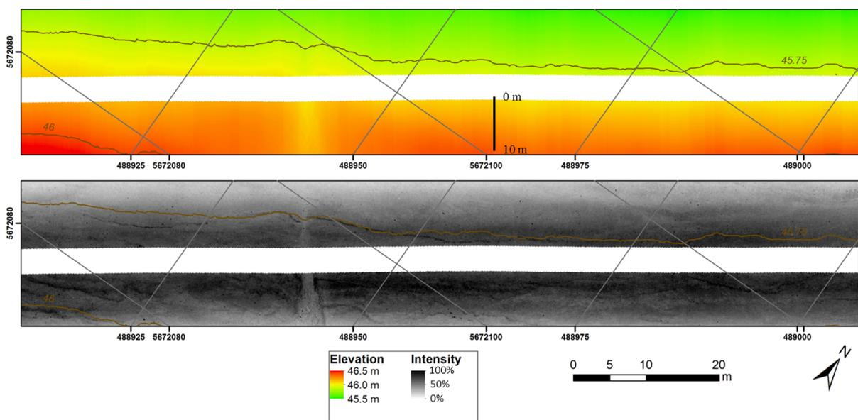
Figure 7: Elevation map (top) and intensity map (bottom) acquired from the same track line
