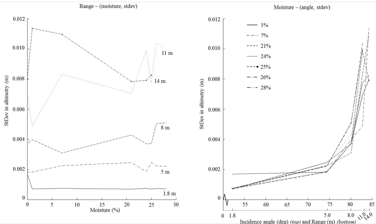
Figure 3: The range in function of the moisture and standard deviation in altimetry (left) and the moisture in function of the incidence angle (or range) and the standard deviation in altimetry (right)
