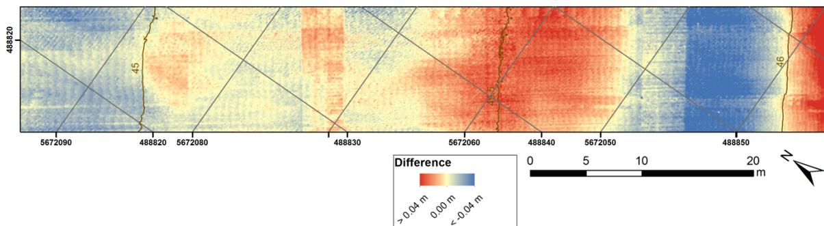
Figure 6: Differences in altimetry between MTLS data and STLS data for the small area on the beach
