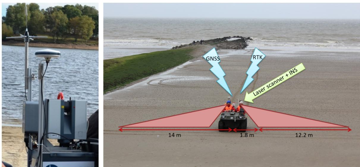
Figure 3 : Side-view of MTLs set up (left) – Performance principle of MTLs method (right)
