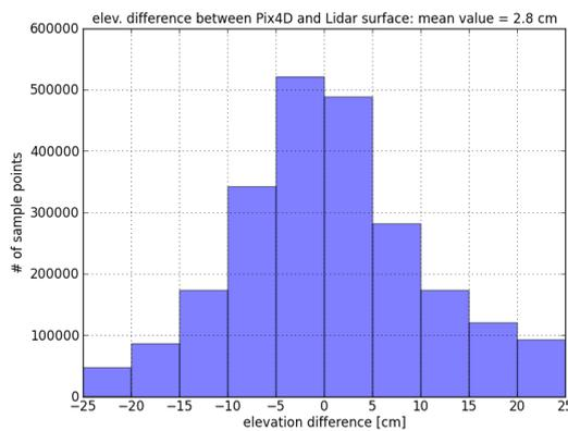
**Figure 5** Elevation difference histogram between LIDAR based surface points and Pix4D DSM surface.
