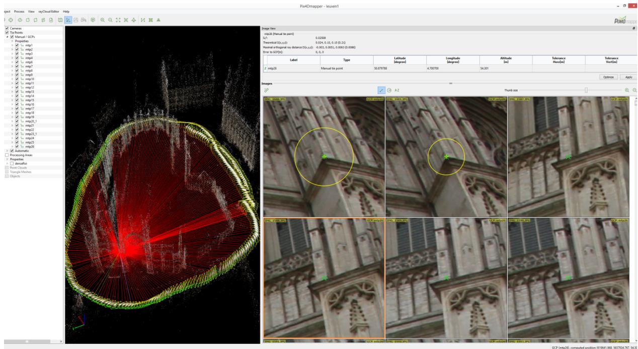
*Figure 3 Pix4D rayCloud: measuring point in stereo.*
