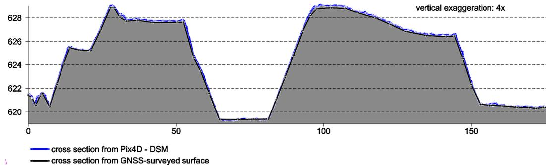
**Figure 7** Comparison of stockpile cross sections between Pix4D DSM and GNSS surveying points.
