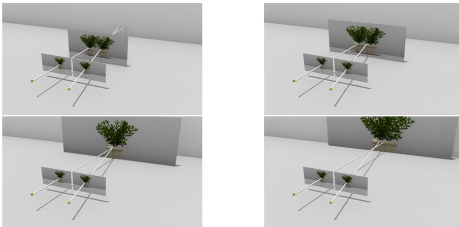
**Figure 1 Stereo measurement by triangulation:** A scene is captured by two images. The knowledge of their respective camera centre allows to obtain a 3D point by finding the corresponding pixels and use them to intersect the two camera rays that go through these pixel locations (left-bottom). Similarly, stereo displays give the user the possibility to move a virtual plane such that the image projections onto that plane coincide.
