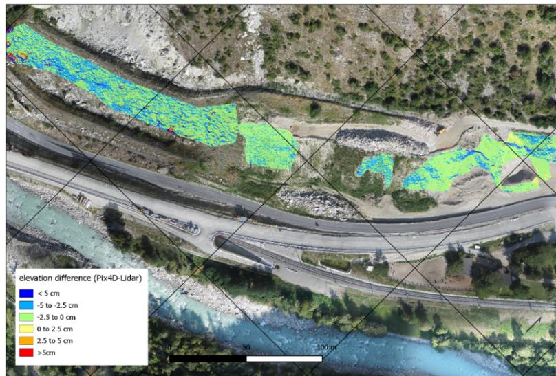
**Figure 6** Top view with colour coded deviation between LIDAR survey zones and Pix4D DSM.
