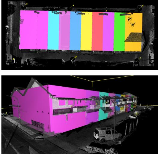
Figure 9: Boundary lines are extruded into 3D boxes and shaded in different colors to represent every different lot. (Above) Top view & (below) perspective view.
