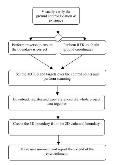
Figure 6: The general workflow of TLS in encroachment detection.
