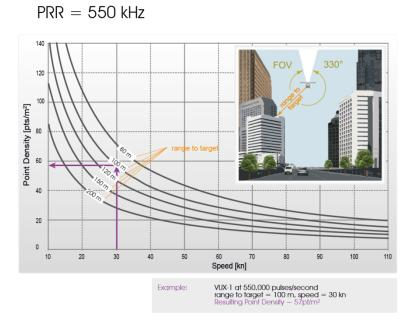
Fig. 4: Performance envelope-2, 550 kHz
