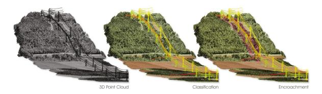
Fig. 11: Power Line Inspection
