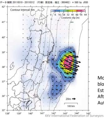
Model of co-seismic slip of upper block against descending slab Estimated from GPS data After Geospatial Information Authority and Japan Coast Guard
