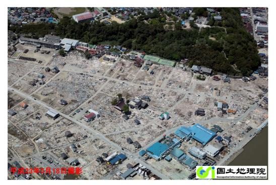
Boundaries of parcels are washed away by Tsunami. If cadastral maps are available, we can recover present position of boundaries in reference to displacement of control stations (after 26SI, Japan)
