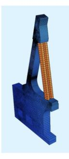
finite element mesh of pylon
