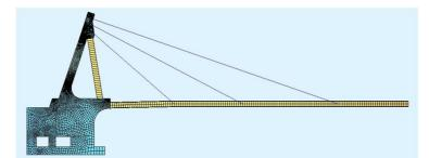
finite element mesh model of bridge
