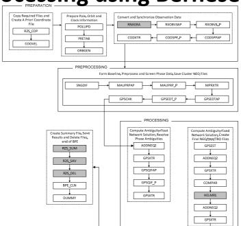
Double difference GPS processing step, 3 parts: preparation, pre-processing and processing
