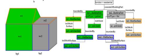
LoD2 building illustration: CityGML feature structure as UML instance diagram
