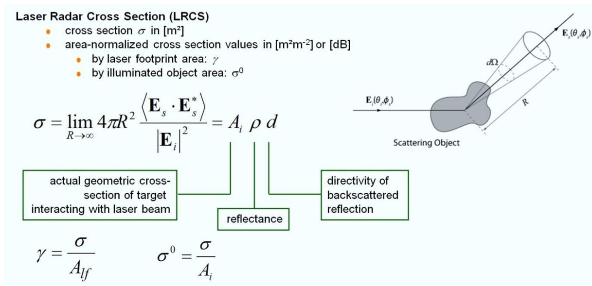
Fig.1 Radiometric calibration of the reflected signal
