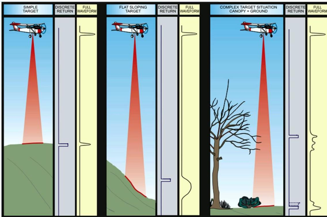
Fig. 3 A single reflected signal in comparison with one, but with a full-wave analysis
