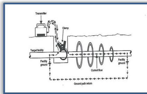
Figure 6: Detection of metallic pipes with EML
