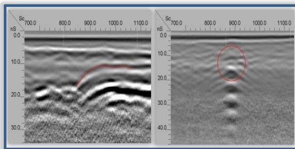
Figure 5: Left profile displays edge of excavation and right profile indicates presence of non-metallic utility pipes
