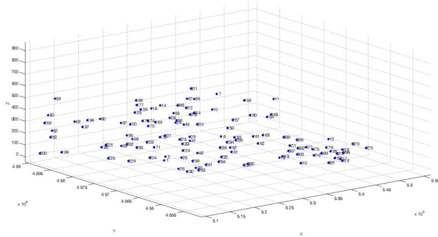
Figure 1. The Samsun triangulation network
