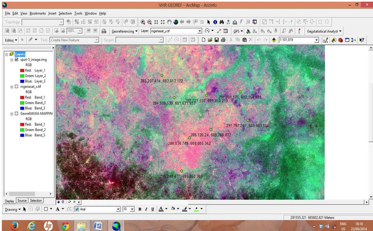
Fig.4 HIGH RESOLUTION IMAGE OF STUDY AREA SHOWING LOCATION OF CONTROL POINTS (SPOT 5)
